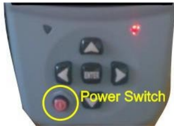
Power switch position
